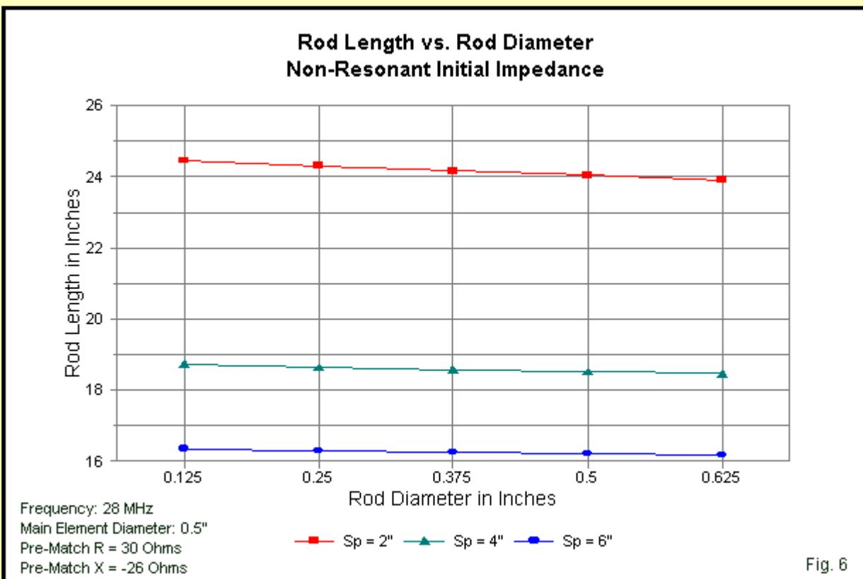
The curves for each spacing increment show a definite "tilt" and become shorter as the gamma rod becomes thicker. However, the amount of length change for the change in the element-to-rod ratio is quite small: a 2% length change for a ratio change of 5:1. This result suggests that one might explore other directions in gamma-match variables by using a single element-to-rod ratio with confidence that the results for other ratios would not jeopardize the validity of the trends uncovered.
