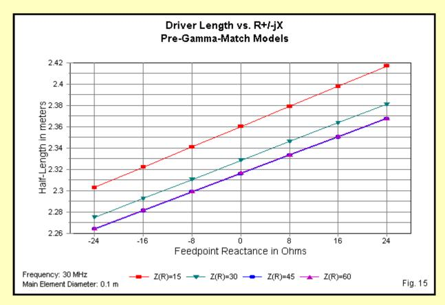
As we saw for the case of resonant initial impedances, there is virtually no difference between the driver lengths for 45 and for 60 Ohms, regardless of the reactance. Indeed, were it not for the slight changes in the resistive component of the initial impedance, the graphed lines might be arithmetically linear.
