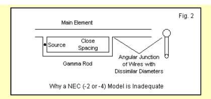
If we were using models with gamma rods that varied in diameter from the main element diameter, NEC would reveal its well known weakness at angular junctions of wires having different diameters. However, the models in this study will use equal diameters for all wires. Nevertheless, with relatively close spacing of wires, NEC also begins to yield errant results, as indicated by average gain test (AGT) scores that depart widely from the ideal value of 1.0000.
