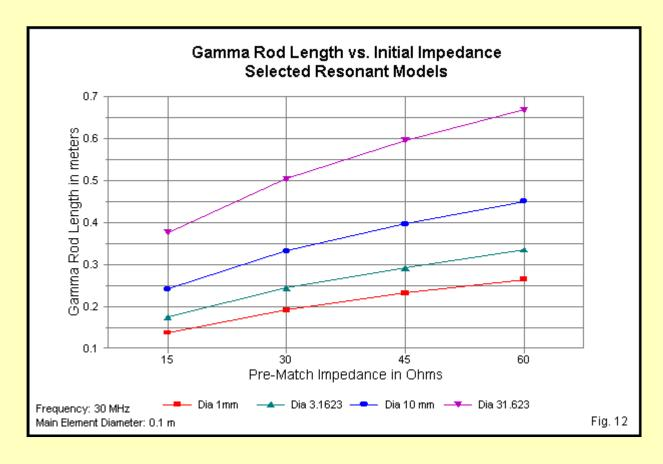
As we increase the element diameter, the curve of gamma lengths becomes steeper, increasing with the initial feedpoint impedance. For each curve, the slope decreases as the initial feedpoint impedance comes closer to the target impedance, although the required length continues to increase. **Table 3** provides a reference table of the data in the graph, re-grouped for easy correlation.
