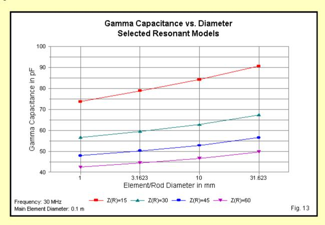
If we re-group the data by element diameters, we can see the degree of required capacitance decrease as we increase the initial feedpoint impedance for all wire diameters. The graph in **Fig. 14** has a quite different appearance than the one in **Fig. 13**, although both graphs cover the same overall data set. Looking at only one of the two graphs might well leave a misimpression of the changes that occur from one step to the next.
