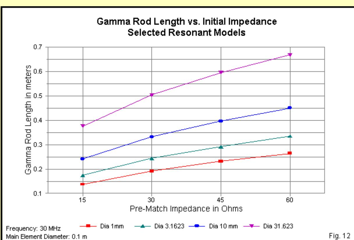
As we increase the element diameter, the curve of gamma lengths becomes steeper, increasing with the initial feedpoint impedance. For each curve, the slope decreases as the initial feedpoint impedance comes closer to the target impedance, although the required length continues to increase. **Table 3** provides a reference table of the data in the graph, re-grouped for easy correlation.
